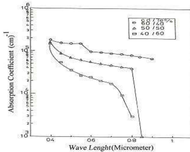
Figure 4: Dependence of Absorption Coefficient on Cd percentage
